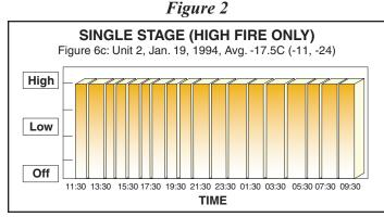
These two graphs, reproduced with permission from the RDM Engineering Report, dramatically demonstrate the operating differences between the two-stage and single-stage input infra-red alternatives.
