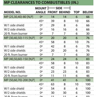
Clearances published in MP Series manual and on warning label supersede data shown on this brochure. Reference MP Series installation manual for complete information.
